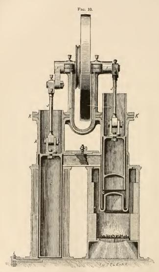
to ascend, the plunger comes down and the operation is repeated. When the air passes from the heater to the cool cylinder A, it heats the plates of the regenerator and this heat is given off to the cool air, when it is again forced into the heater. The utmost of the heat is thus utilized that is possible. The start in this as in all hot-air and gas engines must be made by hand, but after a few turns of the fly-wheel the motion acquired is maintained by the engine.
